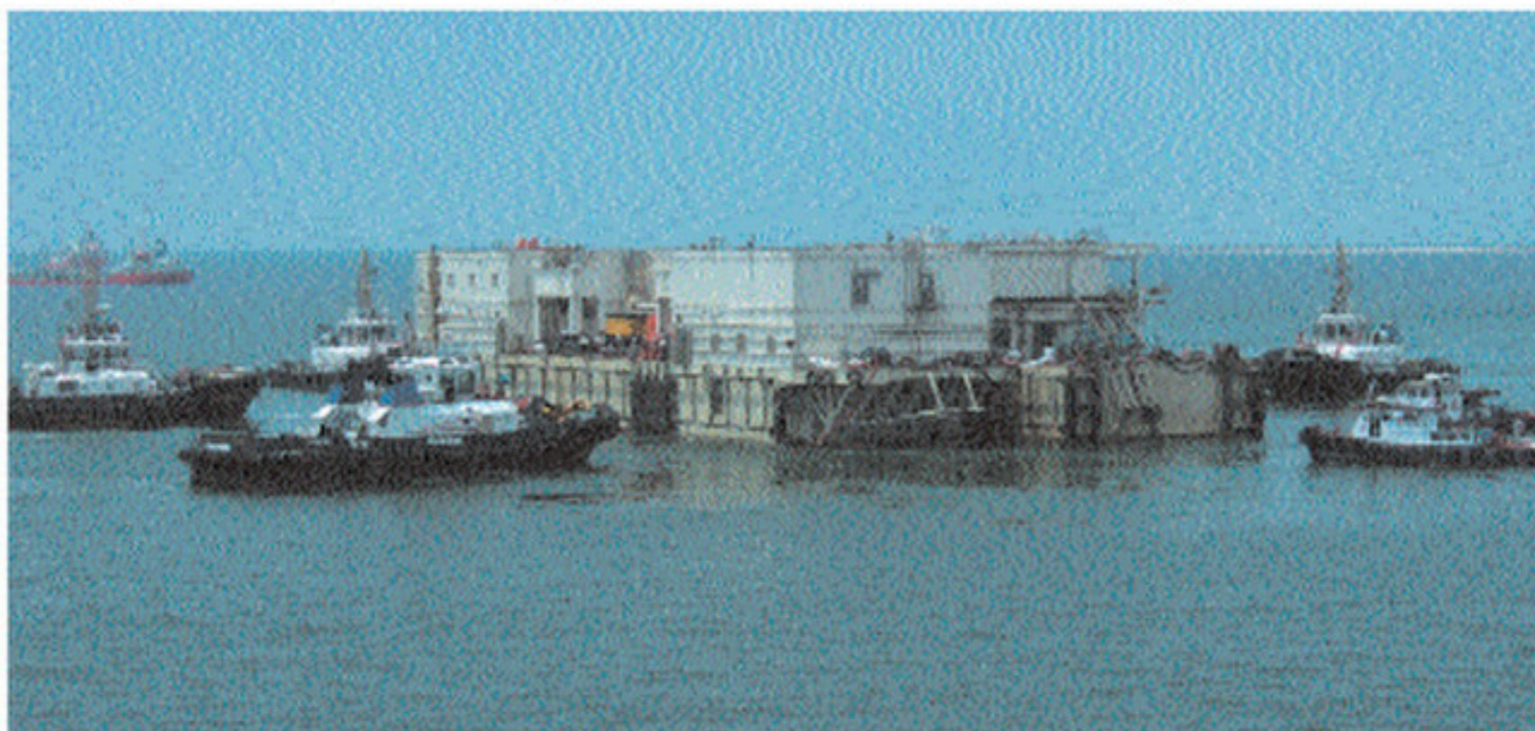
2 of the 4 self-floating modules navigated by 5 tug boats from the shipyard in Singapore heading for the Mighty Servant 3 in the background after loading.
