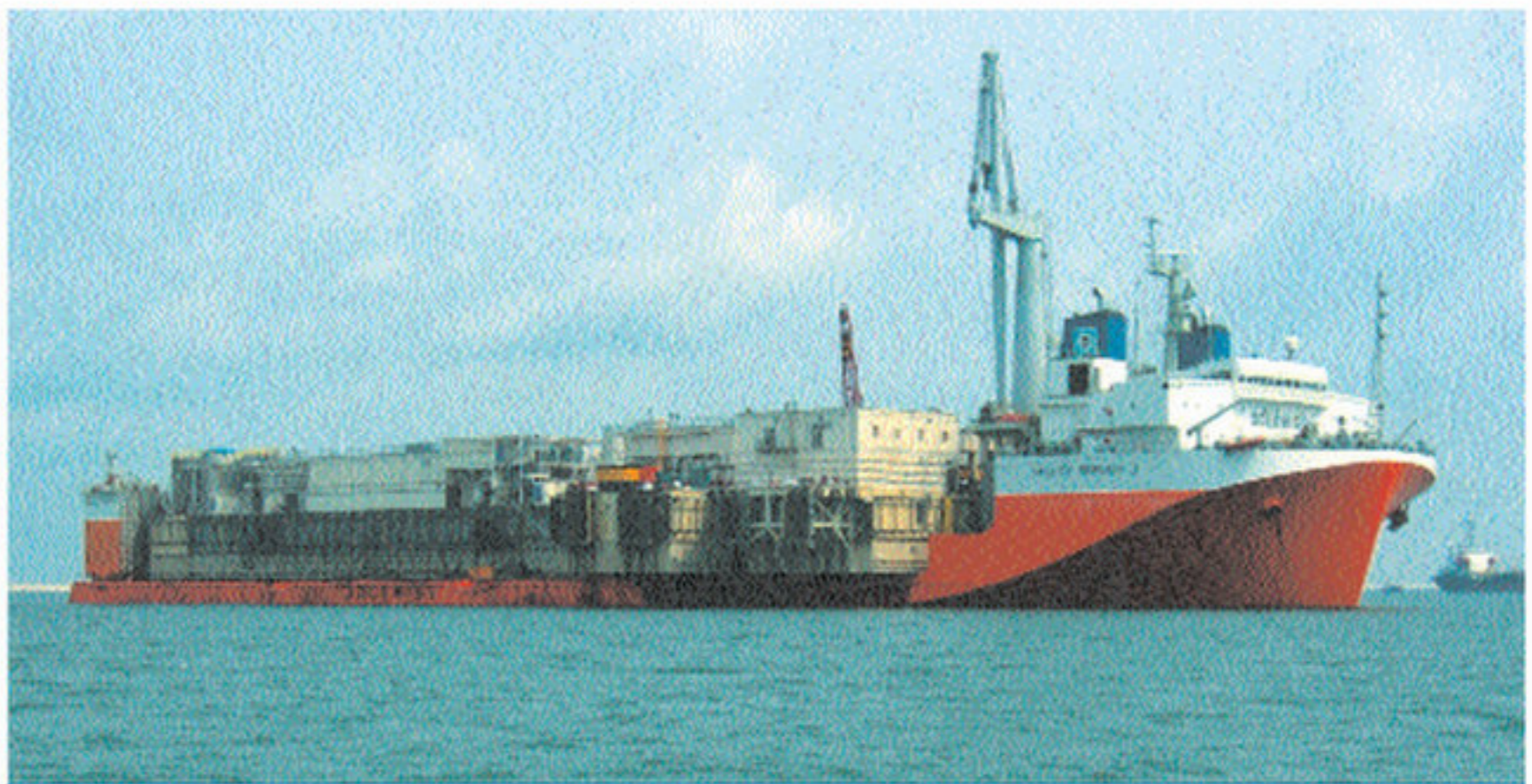
Mighty Servant 3 - loaded with 4 self-floating modules which constitute the main deck of the gas production platform.
