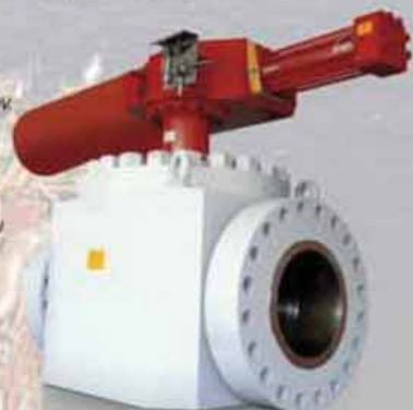
Series BTE Top-entry ball valves. Applications Top-side, ESDV. Pressure classes ASME up to ASME 4500 or up to API 15000. Size from 2" up to 48". Available Materials: low temperature carbon steel, Duplex, exotic material or cladding in Inconel material all welded parts.
