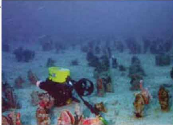
A Fugro eyeball ROV surveys mussel-beds
