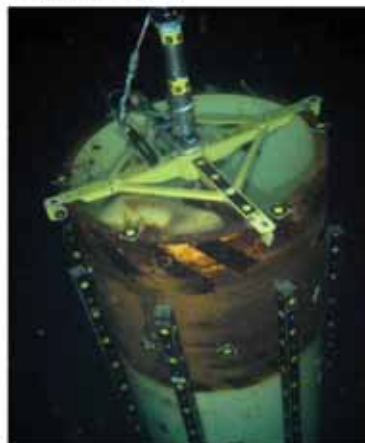
Pin pile with Transponder and photo targets
