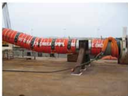
Arrangement of Targets and Target mats on 30" Spool
