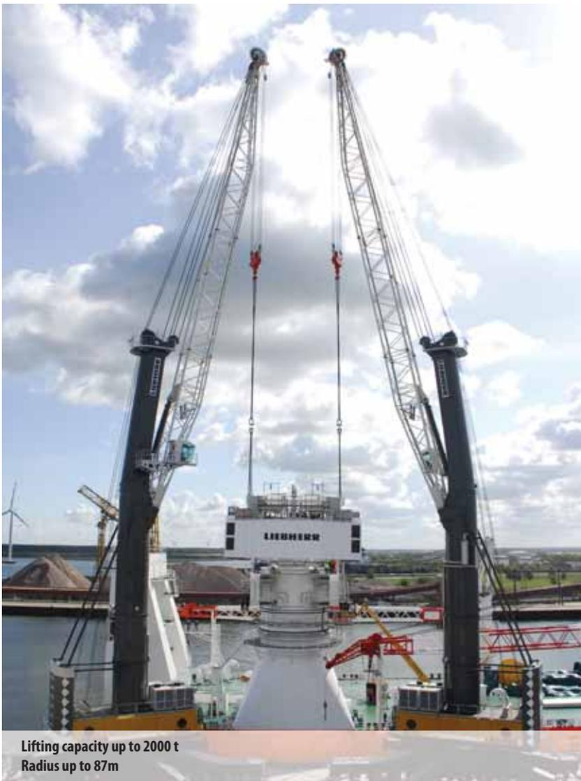
Lifting capacity up to 2000 t
